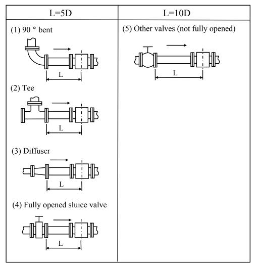
L: Required straight pipe length—straight pipe length plus half length of the detector. D: Nominal bore size (diameter)
